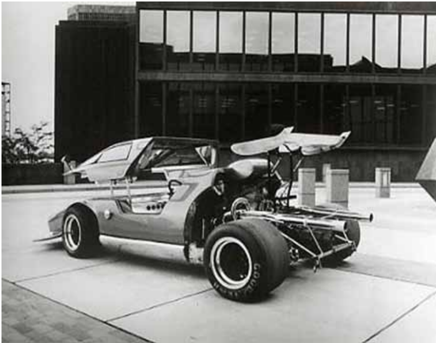
Herb's show car, a custom Lola T-70 with my wing installed at the rear.
